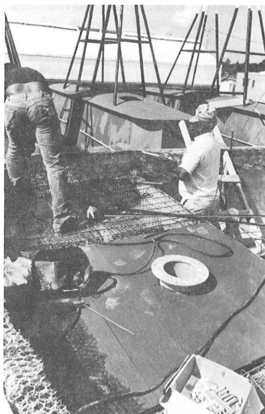
Deck mold over steering compartment.
