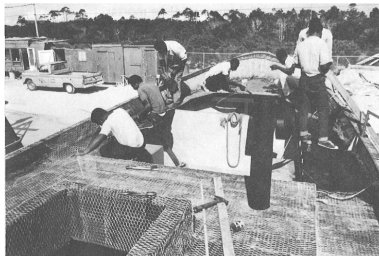
Mesh laid over deck and into fish-hold.
