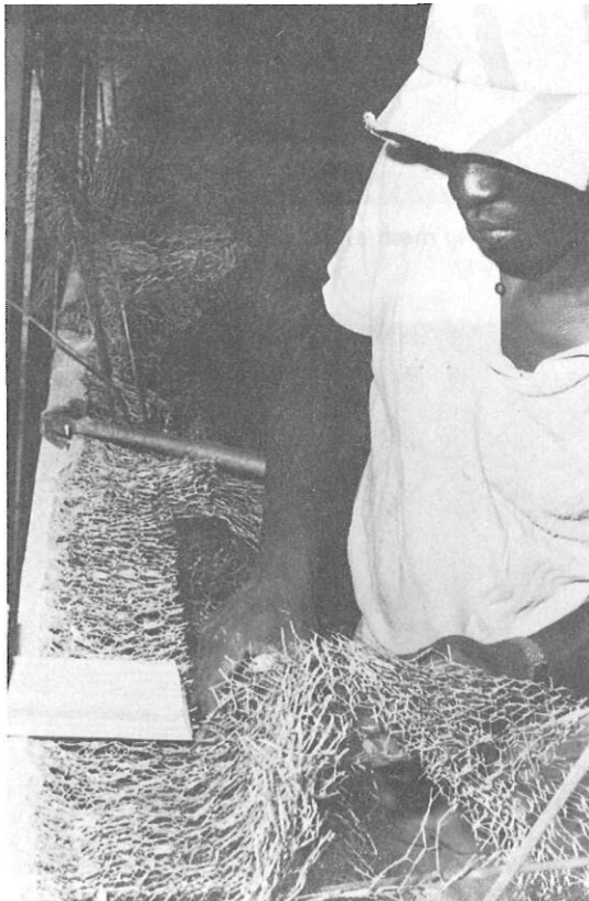
Trimming rail cap mesh. Note wooden guide.
