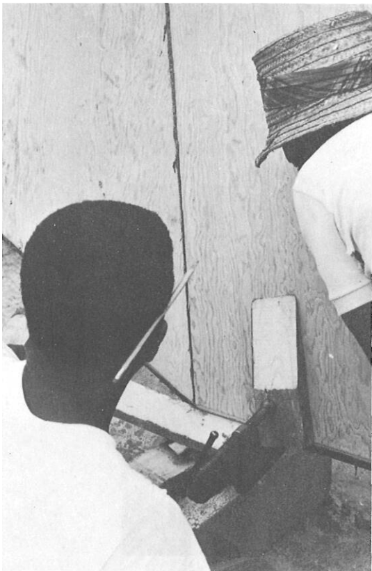
Bottom round edge of plywood is raised above deck level.
