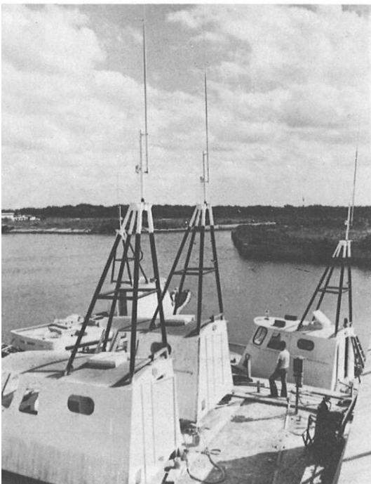
Masthead assemblies welded into place.
