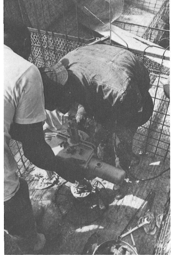
Hydraulic steering mechanism packed with grease.
