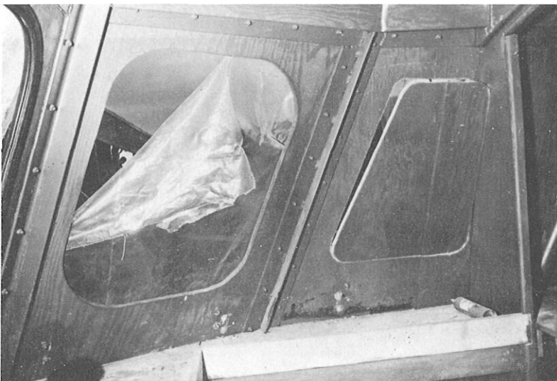
Window corners are well rounded for the fitting of rubber molding.
