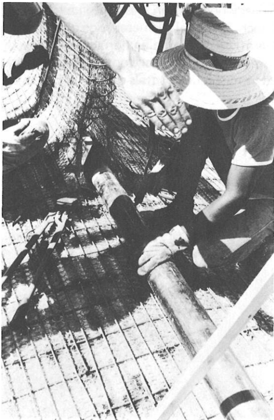
A hole is cut in the keel reinforcing.
