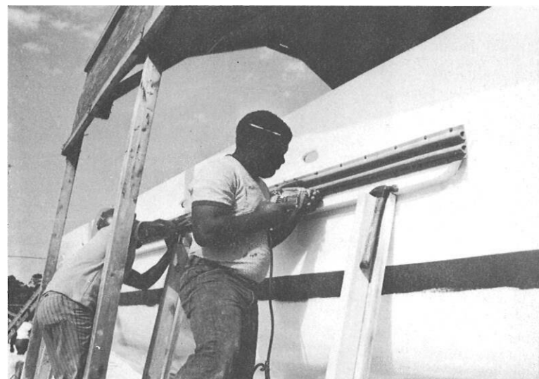
Fastening rubber fenders to the rubbing strakes.
