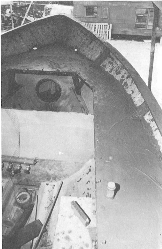
Note wooden plugs to superstructure bolt-holes, fuel tank filler cap.
