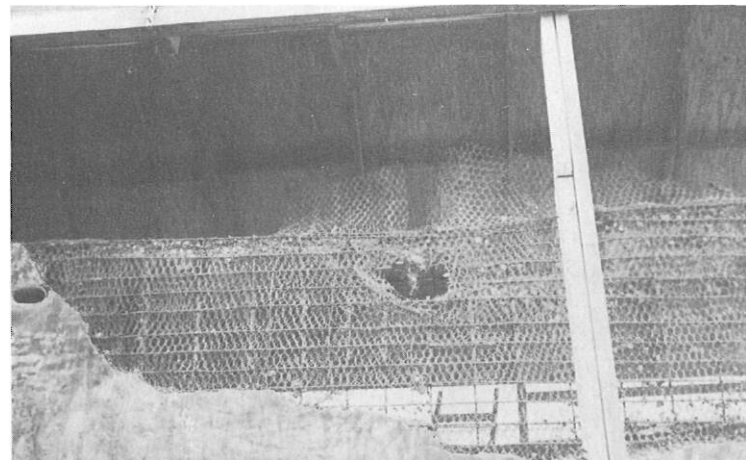
View from outside of the hull damaged when dropped on its side.
