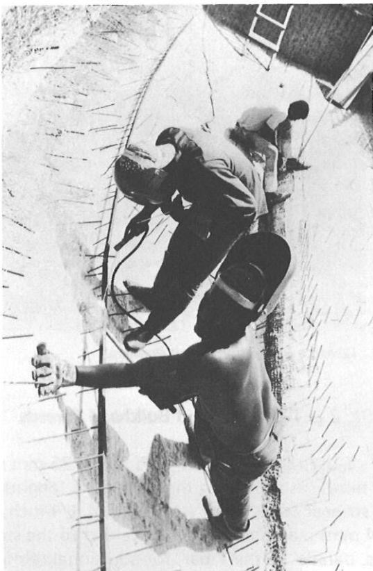
Welding T-bar screed to bilge stringer starter rod.
