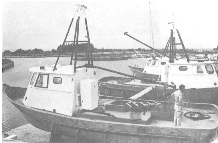
"Seafarer" ice machine installed with fiberglass cover.
