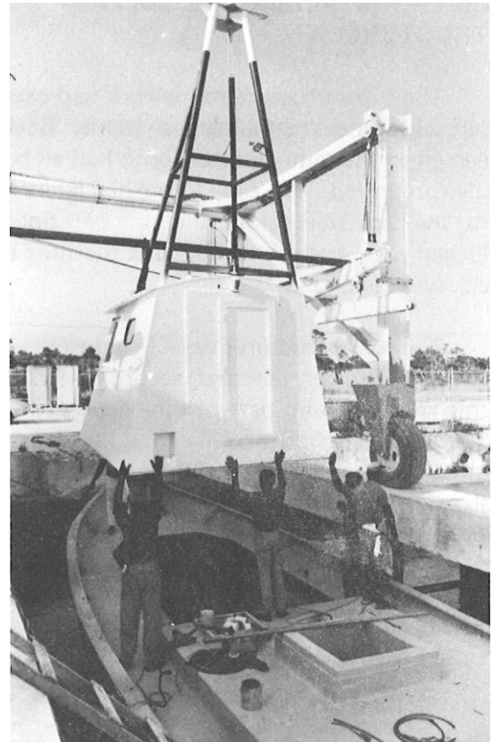
Comporter lowering superstructure onto a hull afloat.
