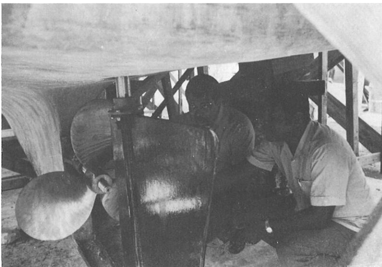
Two-piece rudder stock bolted together and the rudder assembly in place.
