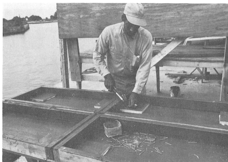
Hatch interior primed; hinge butt blocks fastened.
