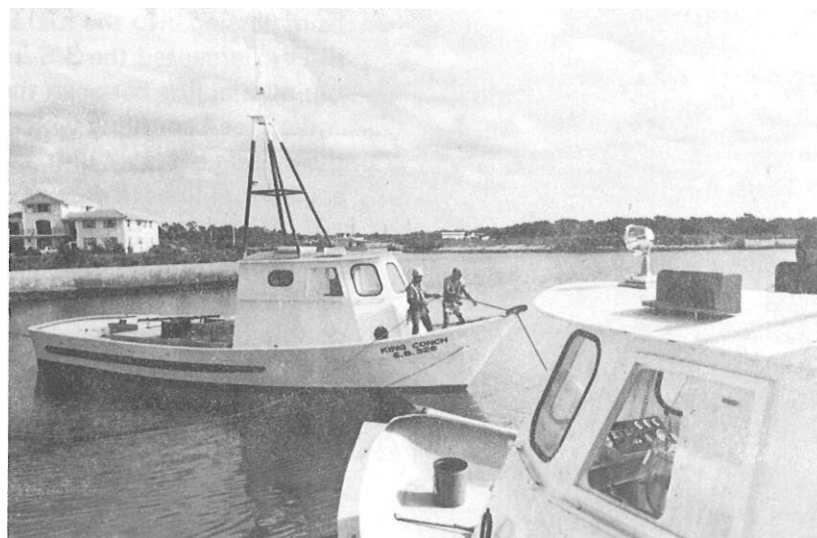
Another boat is launched and warped alongside for final out-fitting.
