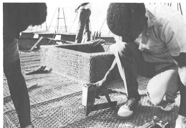
Stapling deck reinforcing rods athwartships.
