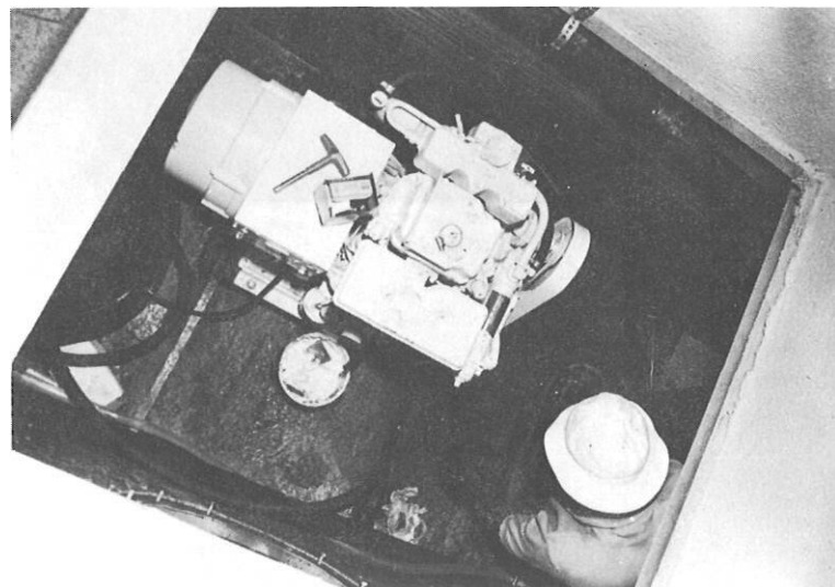
Installing the diesel generator unit in the lazarette.
