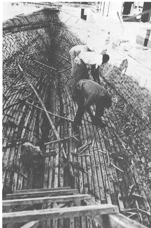
The strippers work from the sheer downwards.
