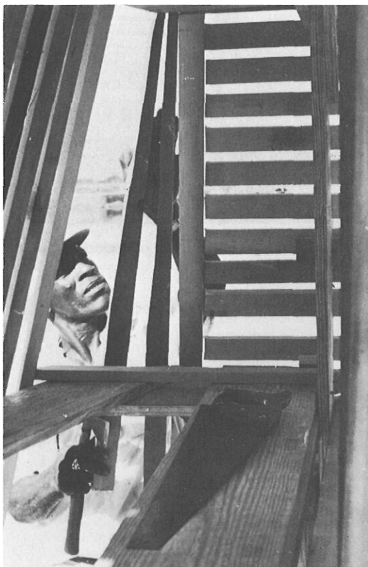
Tapering planks for transom mold.
