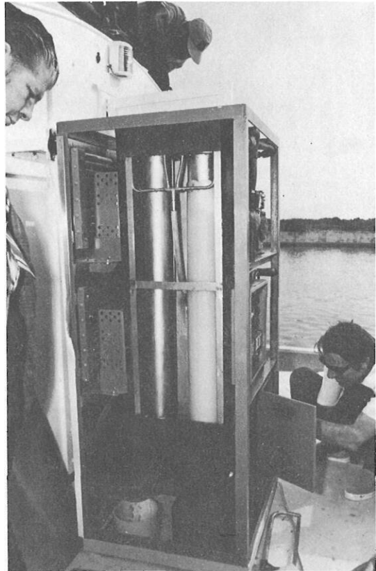
Checking the seawater ice machine installation. The first nickel-plated evaporator cylinder has just harvested its ice, the second is following.
