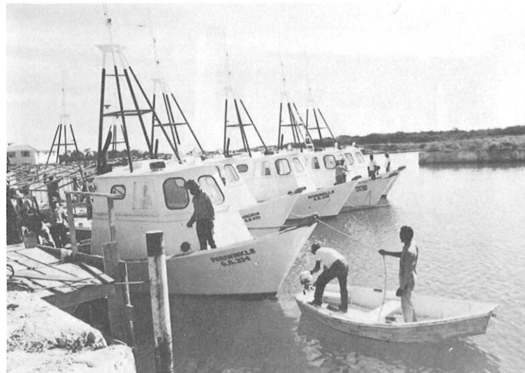
Fiberglass radio antennas fitted to topmasts.
