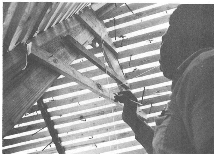
Propeller shaft center line is extended to the bow for accurate alignment.
