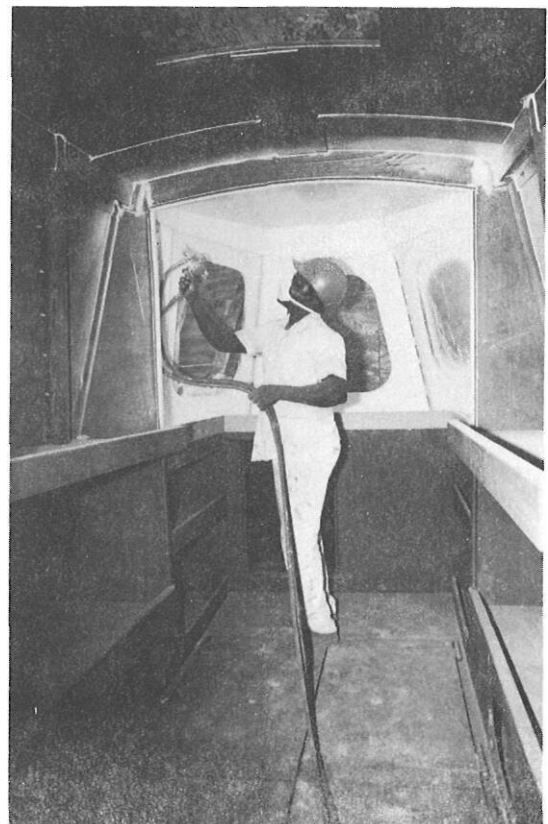
White enamel spray paint finish for the interior.
