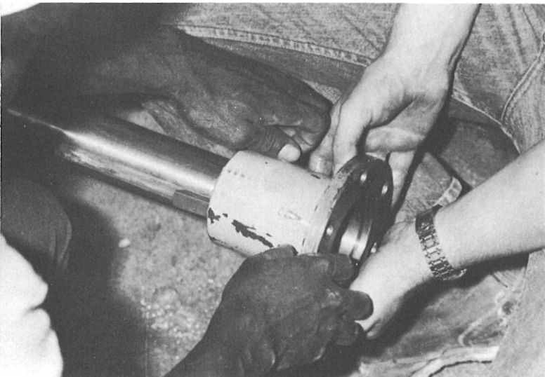
Fitting propeller shaft half coupling.
