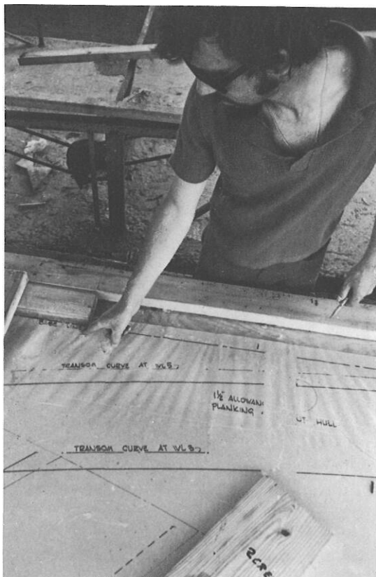
All hull mold frames measure from this Base Line.
