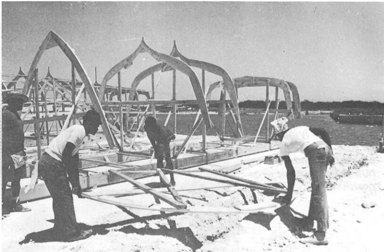
Handling the hull mold frames with care.
