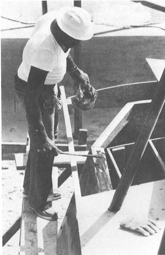
Bedding compound spread over topside packing.
