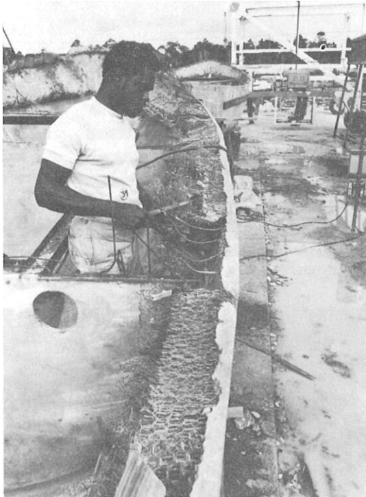
Cutting rail cap rods to length.
