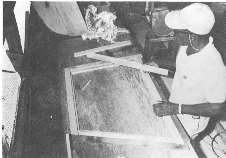
Sliding window frames in the jig.
