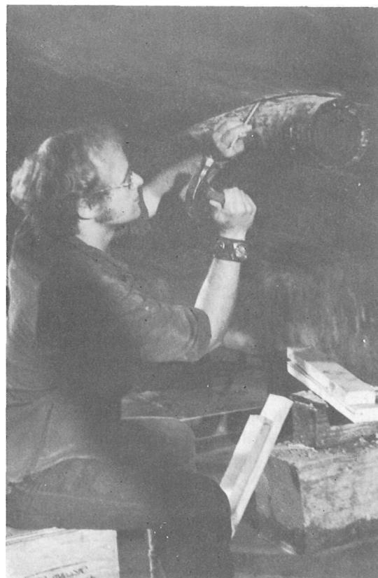
Calking shaft log aperture.
