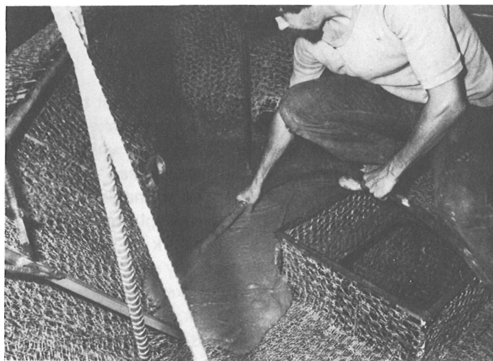
Start applying mortar to the deck at the stem.
