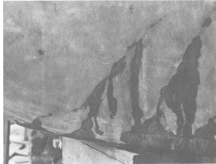
Crane-dropped hull showing damage, cracks leaking and sealing with sodium silicate.
