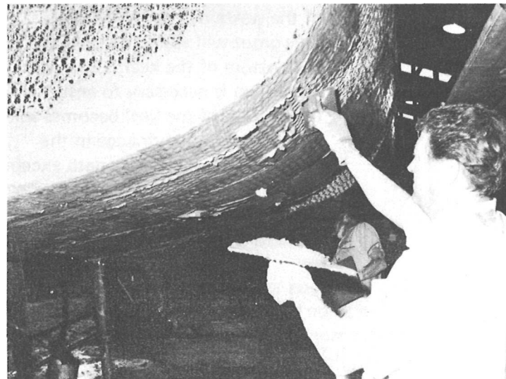
A plasterer punching the mortar against the hull.
