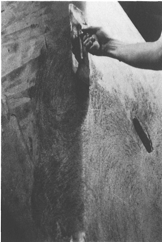
The swimming pool trowel is used for finishing work. Here the hull has just been sponge-floated and the plasterer is now starting the first part of steel troweling.
