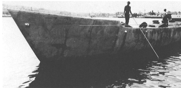
The careful use of screeds in fairing the hull sheer is justified when the vessel is seen on the water.
