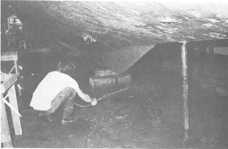
On a hot day spray water under the hull to stop flash setting.
