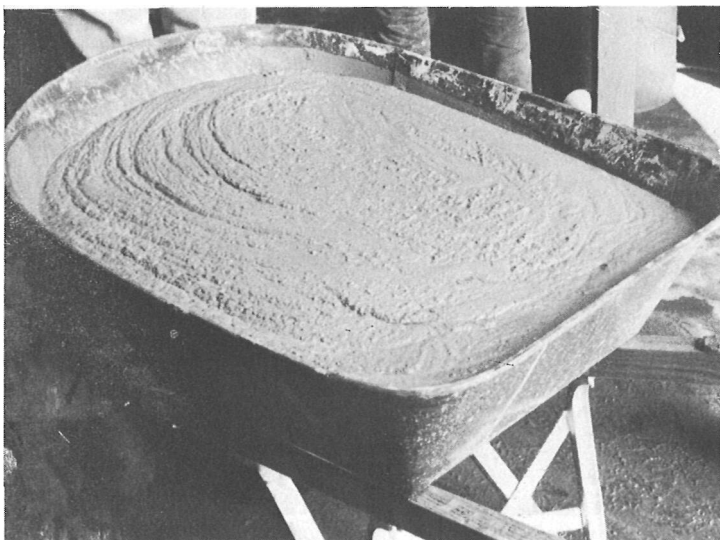
A wetter mix to be used over a mold.
