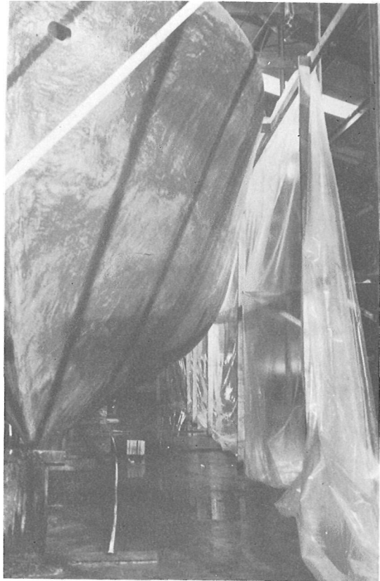
Keep plastic clear of the hull.
