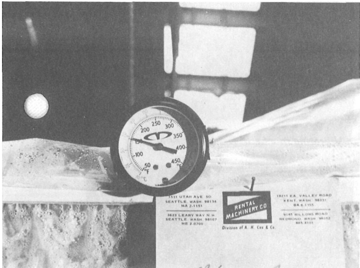
Thermometers reaching into the hull to register hull temperature at various points.
