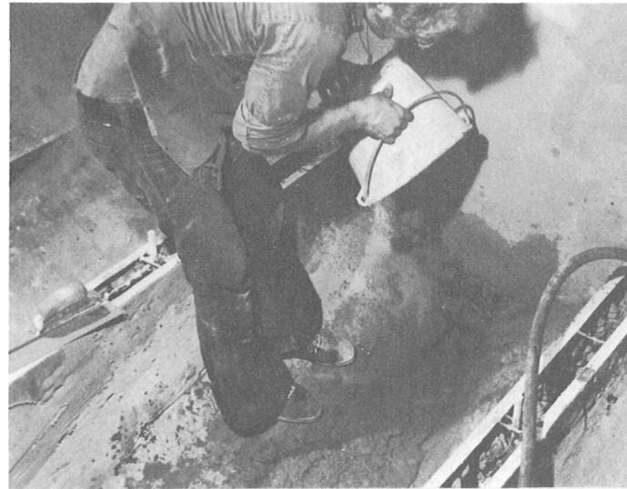
Mortar is dumped into keel bottom.
